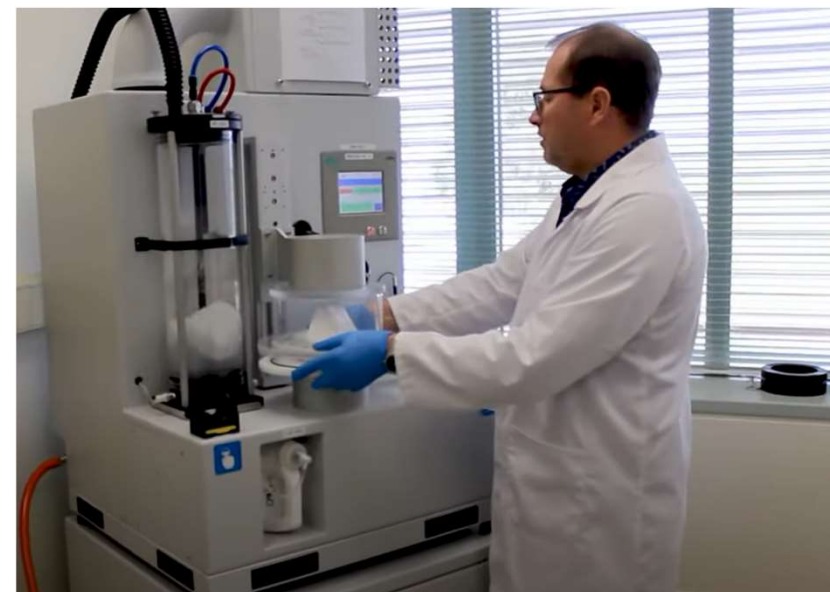
TGA officer testing the particulate filtration efficiency of a N95 respirator
